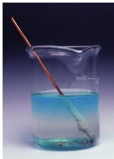
fig A The photo shows what happens when a copper wire is placed in silver nitrate solution for some time. You can see the results of the displacement reaction, the 'growth' on the wire is silver metal and the blue solution contains the copper(II) nitrate that is formed.
