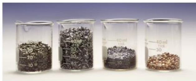
fig A From left to right: tin (Sn), magnesium (Mg), iodine (I) and copper (Cu). Each sample contains 6.02 \times 10^{23} atoms.
